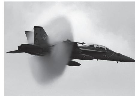
2. A sonic boom produced by an aircraft moving at  $M=2.92$ , calculated from the cone angle of 20 degrees. An observer hears the boom when the shock wave, on the edges of the cone, crosses his or her location.
